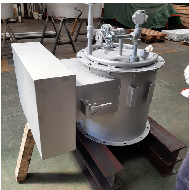
Burner 3D view (base plate)
